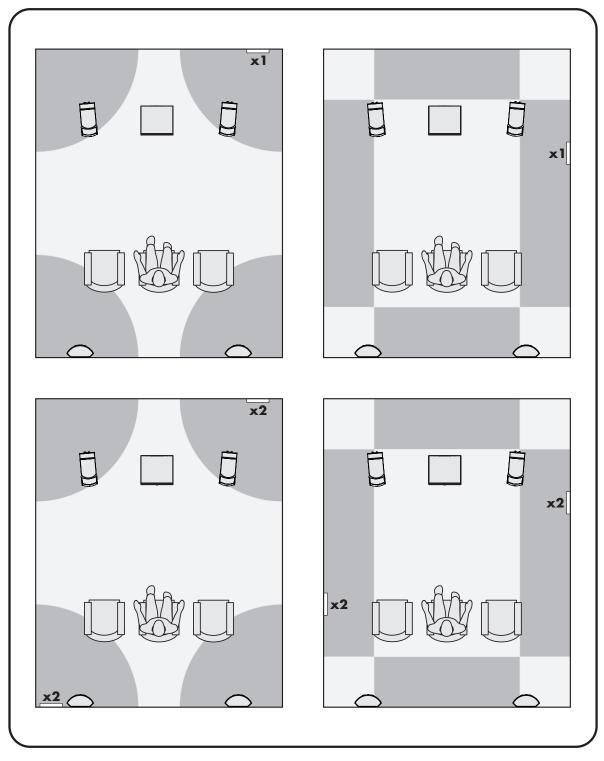
**Figure 6.** Typical Subwoofer placement options indicated by the shaded areas. Your unique room design may require another alternative.
