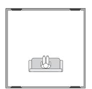
Fig. 1c Recommended placement for four subwoofers
