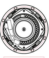
CUTOUT DIAMETER (WITH TOLERANCE) 7.75in [196mm]
