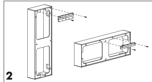
Attach (1) bracket to the back of the On-Wall Frame in the desired orientation using (2) screws. Please Note: Attaching the bracket to the Monument 7XW On-Wall Frame in the horizontal orientation will require (3) screws.
