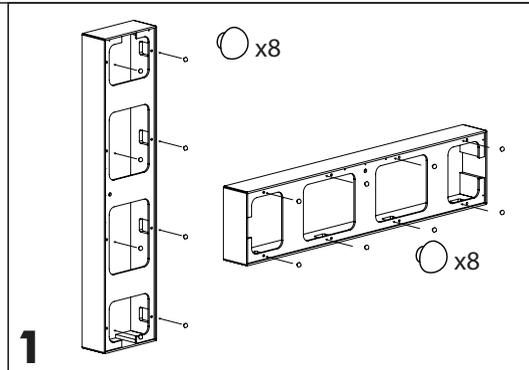
The Monument 7XW On-Wall Frame can be used in either a vertical or horizontal orientation. (8) rubber bumpers need to be installed on the back of the frame when used in either orientation. These bumpers are designed to help protect the wall finish and help eliminate any unwanted noise caused by surface to surface contact between the frame and wall.
