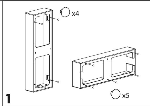
The Icon 3XW and Tribute 5XW On-Wall Frame can be used in either a vertical or horizontal orientation. (4) rubber bumpers need to be installed on the back of the frame when used in a vertical layout, and (5) bumpers will be required when used horizontally. These bumpers are designed to help protect the wall finish and help eliminate any unwanted noise caused by surface to surface contact between the frame and wall.
