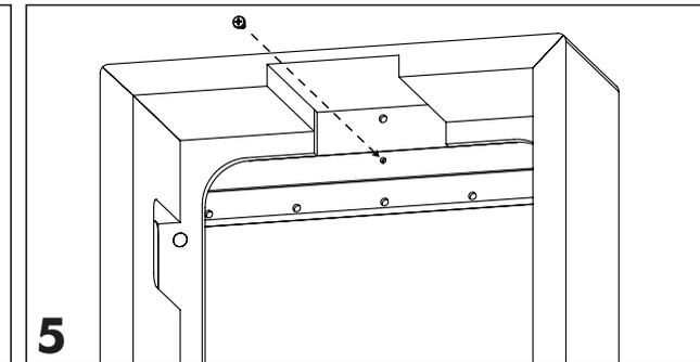
Insert (1) included sheet metal screw through the hole in the bracket to secure the frame to the wall.
